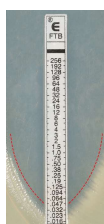
Figure 1 E. coli ATCC 25922 MIC = 0.047 \mu g/mL Read at complete inhibition of haze
